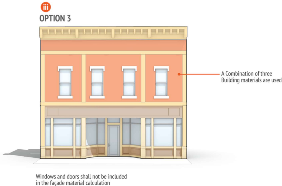
Figure 7 - Exterior Building Cladding Materials, Option 3
