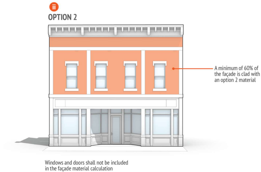
Figure 6 - Exterior Building Cladding Materials, Option 2
