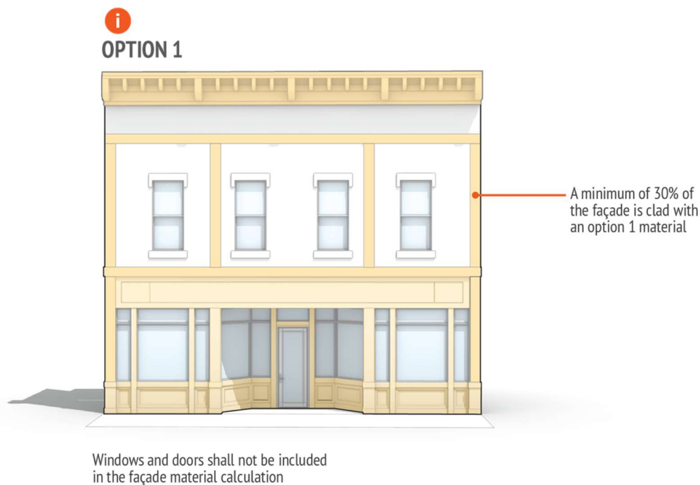
Figure 5 - Exterior Building Cladding Materials, Option 1
